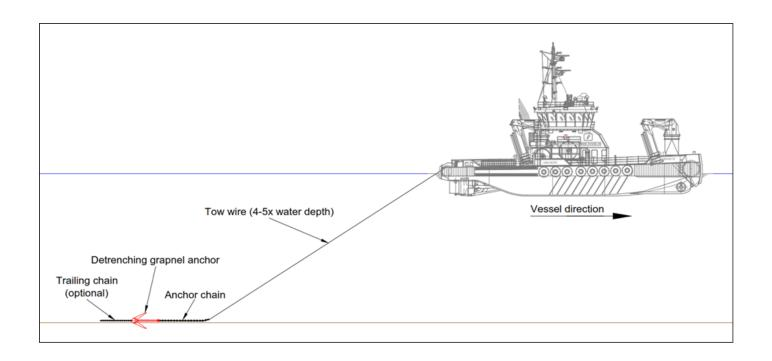
The De-Trenching equipment consists of several components, which are listed on the following page
